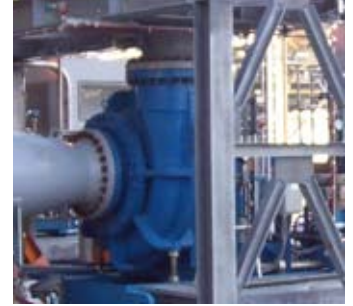
Hazleton CTC 20-30 with 20" suction and discharge
